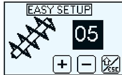
If you notice an excessive deposit on the burner pot, enter the EASY SETUP program and lower the value by one unit to “- 1”; then wait for the following day and if there is no improvement, lower the value again up to a maximum of “- 3”. Instead, should it be necessary to increase the calibration of the volumetric weight of the pellet, it is advisable to go from the default value “0” to “+ 1, + 2, + 3” as required.
