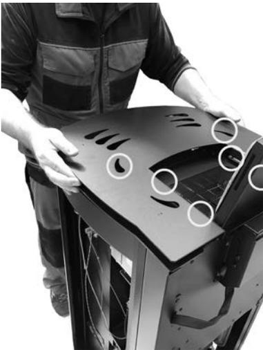
*Fig. 51 - Remove the cover*
