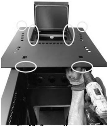
Fig. 57 - Remove the screws
