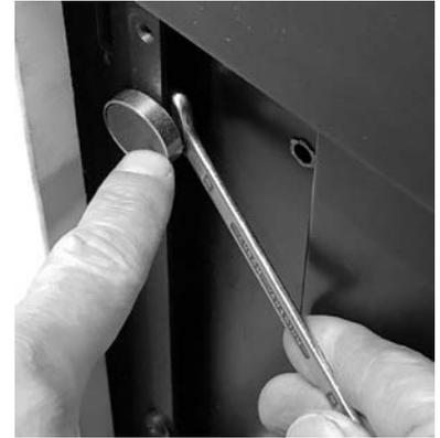
**Fig. 41 - Adjust the magnet and block with the key**
