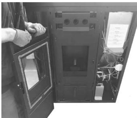
**Fig. 45 - Remove the door**
