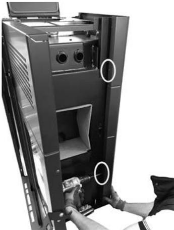
Fig. 59 - Secure the front side panel
