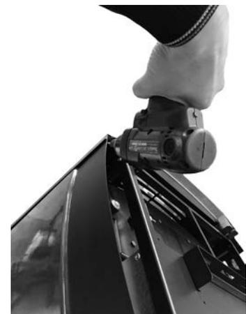
*Fig. 56 - Fasten the compensator*
