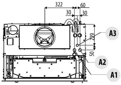
Fig. 20 - Connection diagram SATURNO
