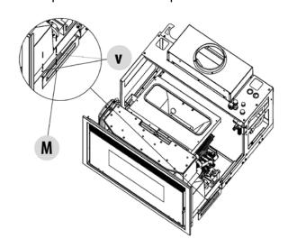
• the handles "M" are now fastened on the insert. Hold the two handles "M" and lift the insert
