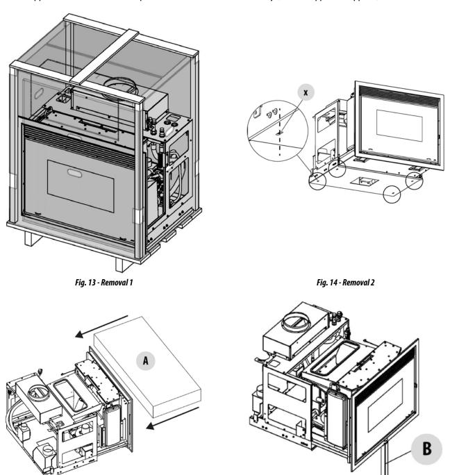
The appliance must always be carried upright, taking care with its moving parts. Pay particular attention to the door and its glass, protecting them from mechanical impact that would compromise their integrity.
