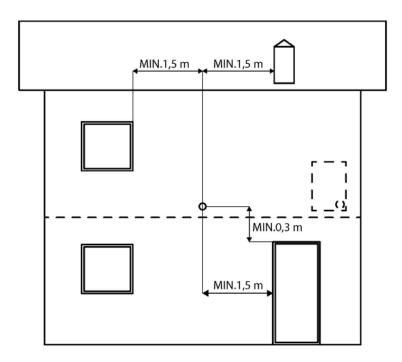
Fig. 11 - Air inlet for sealed-chamber installation
