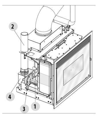
The flue connection is housed, with its ash collection compartment (4), on the rear/side of the product, where the fan outlet is located. Also clean this compartment with a vacuum cleaner by inserting the nozzle on the fan inlet hole.
