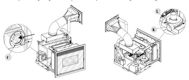
It is also advisable to vacuum near to the coupling "r" and "k" and remove and clean the smoke fan "L".
