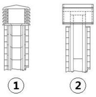
Fig. 4 - Anti-wind chimney pots
