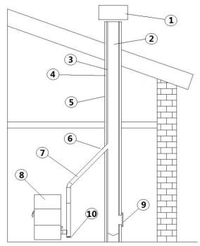
Fig. 5 - Chimney components
