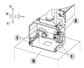
For installation on an existing surface, ensure there is a thickness of at least 17 mm between the fixed wall "A" and the existing surface "U", and fix the insert and surface using plugs "t" as shown on the previous page. Make sure everything is level.
