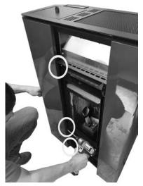
Fig. 47 - Screw removal 3
