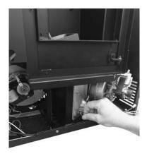
Fig. 64 - Remove the inspection cap
