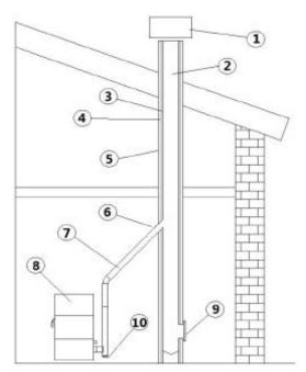
Fig. 5 - Chimney components
