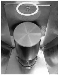
Fig. 74 - Remove the screw
