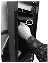
Fig. 67 - Remove screw 2
