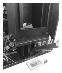
Fig. 65 - Vacuum out the ash
