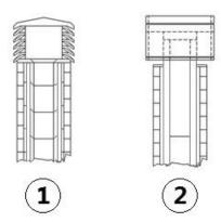
Fig. 4 - Anti-wind chimney pots
