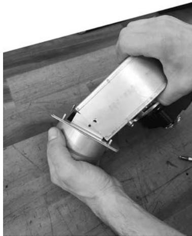
**Fig. 24 - Fix the flange + fitting to the fan**
