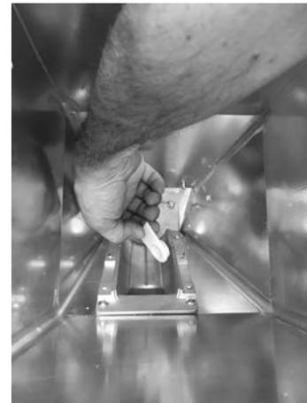
*Fig. 48 - Bearing removal*
