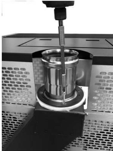
**Fig. 34 - Unscrewing the exhaust**
