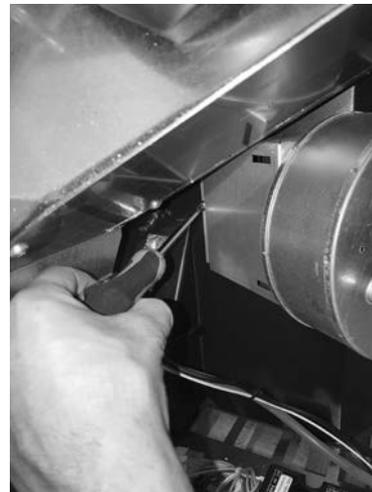
**Fig. 22 - Remove the screw**
