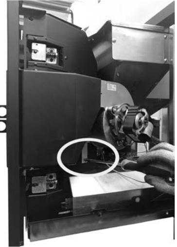
**Fig. 51 - Remove screw 2**
