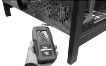
Fig. 42 - Frame<sup>3</sup> digital pressure switch connection
