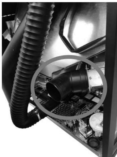
**Fig. 30 - Position fitting at 45°**
