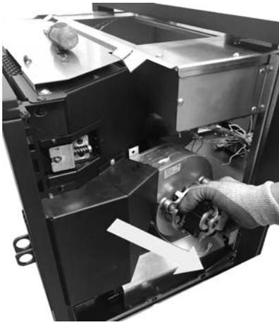
**Fig. 52 - Remove the fan**
