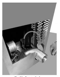
Fig. 73 - Rotate the hose
