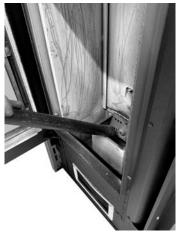
Fig. 92 - Vacuum out the ash
