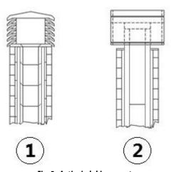
Fig. 5 - Anti-wind chimney pots
