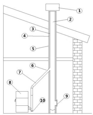
Fig. 6 - Chimney components
