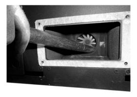
Fig. 107 - Vacuum out the ash
