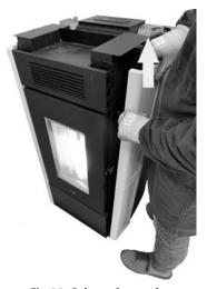
Fig. 35 - Release the panel
