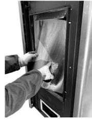
Fig. 101 - Remove the back panel of the firebox
