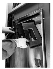
Fig. 99 - Remove the head of the firebox 2
