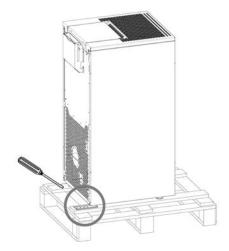
Fig. 1 - Bracket removal
