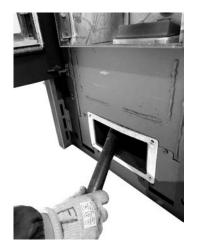
Fig. 103 - Vacuum out the ash
