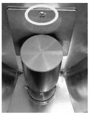
Fig. 112 - Remove the screw
