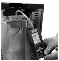
Fig. 89 - Digital pressure switch connection (Atena³ Plus 12/14 - Duke 12/14 At - Saba 12/14)
