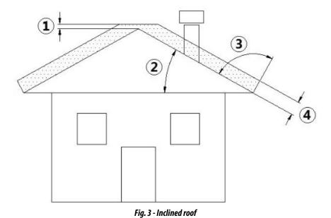
**Fig. 3**Height over the ridge of the roof = 0.5 mt
