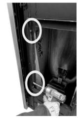
Fig. 97 - Remove the hex screws
