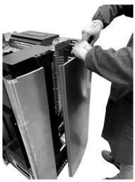
Fig. 29 - Remove the side panels
