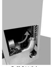
Fig. 80 - Rotate the hose
