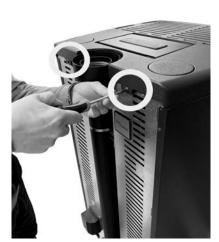
Fig. 20 - Remove the screws
