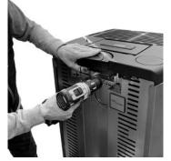
Fig. 49 - Remove the cap (Atena³ Plus 12/14 - Duke At)
