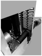
Fig. 78 - Connect the ducting pipe
