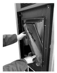
Fig. 100 - Remove the side walls
