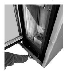
Fig. 30 - Remove the front panels
