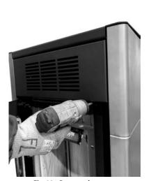
Fig. 23 - Remove the screws
