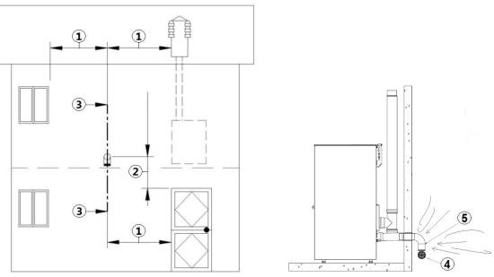
Fig. 10 - Air inlet for sealed-chamber installation
