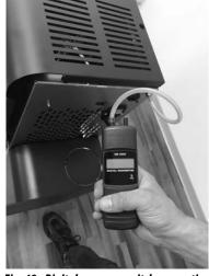
Fig. 48 - Digital pressure switch connection
