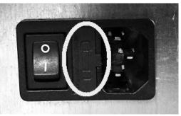
Fig. 49 - Shutter with fuses to remove
