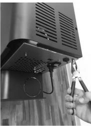
Fig. 47 - Casing removal
