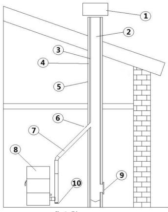
Fig. 5 - Chimney components
