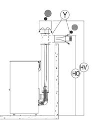
Fig. 15 - Flue connections
