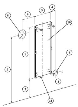
Fig. 24 - Mounting on non-flammable wall
