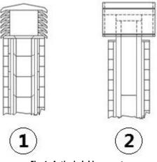
Fig. 4 - Anti-wind chimney pots
