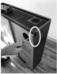
Fig. 35 - Secure the screws
