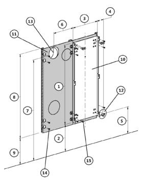
Fig. 25 - Mounting on flammable wall
