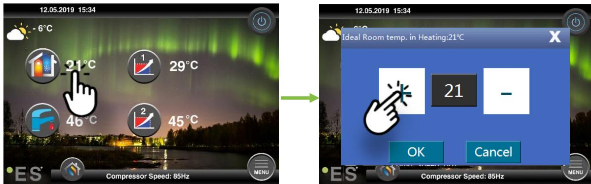
If the window that comes up shows **Ideal room temp. in heating** the room sensor is installed and the heat pump makes small adjustments to the heating curve to keep the desired room temperature.
