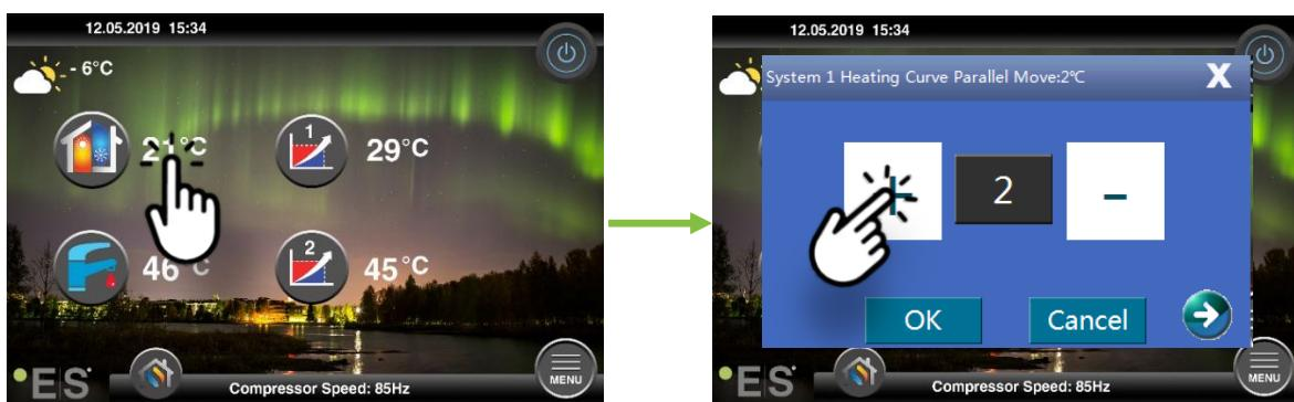
If the window that appears shows **System 1 heating curve para...** the room sensor is not installed or activated. The room temperature is then controlled according to the heating curve.
